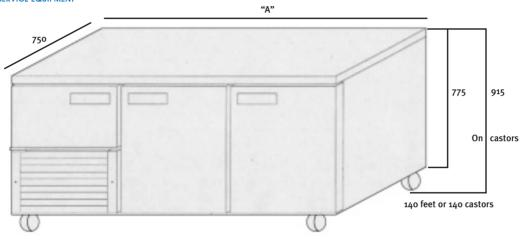
DIMENSIONS "A" - 2<sup>1</sup>/<sub>2</sub> DOOR - 1780mm - 3<sup>1</sup>/<sub>2</sub> DOOR - 2380mm
